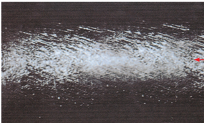
b. 熱浸鍍鋅鋼板在 OT 彎曲試驗中鍍層表面有裂痕現象 Hot-dip galvanized steel exhibits flaking on the coating surface at zero T bend.
