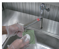
A.3 Clean the specimen with water and gauze it after cooling.
