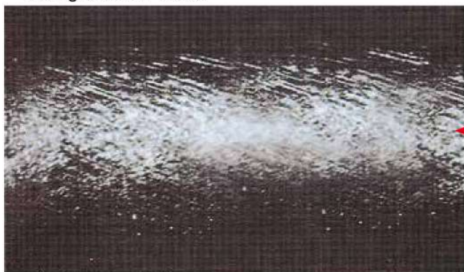
b. 熱浸鍍鋅鋼板 (GI) 在 0T 彎曲試驗中鍍層表面有裂痕現象 Hot-dip galvanized steel (GI) exhibits flaking on the coating surface at zero T bend.
