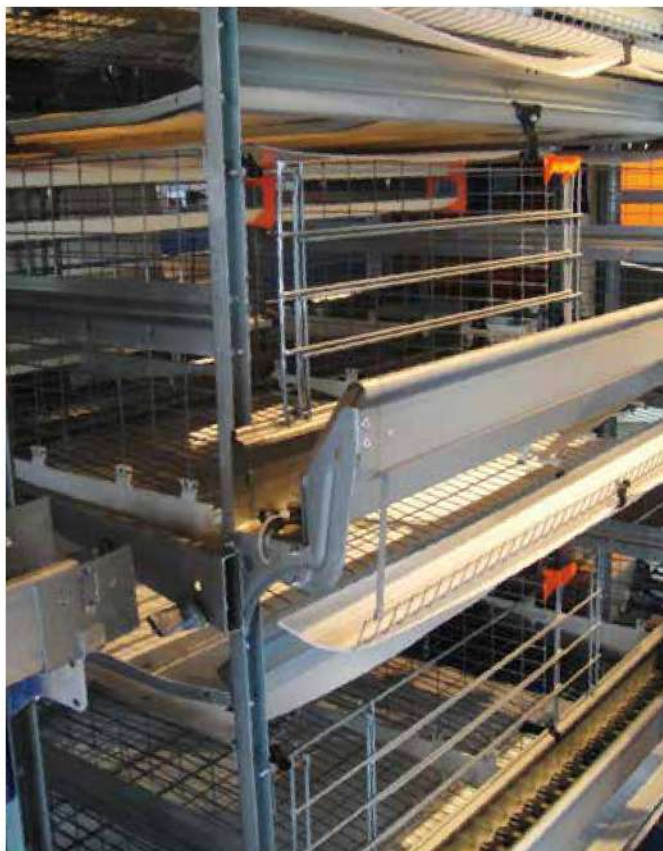
家禽飼餵系統，鍍層量 Y35 Poultry trough Coating mass: Y35
