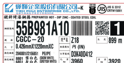
燁輝烤漆產品之標籤示範 Yieh Phui sample of product ID label for pre-painted metallic coated steel coil
