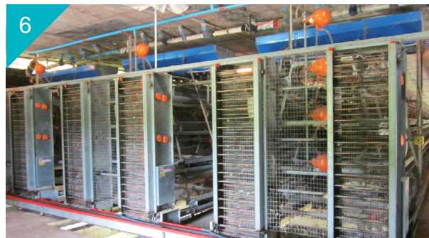
6 自動化禽畜養殖設施用料，熱浸鍍 5% 鋁鋅鋼板 Frame of an automatic poultry feeding system Hot-Dip 5% Al-Zn Coated Steel Sheet
