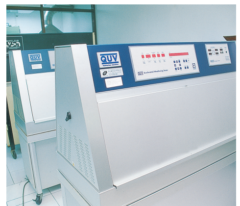
紫外線加速耐候試驗機 QUV Accelerated Weathering Tester
