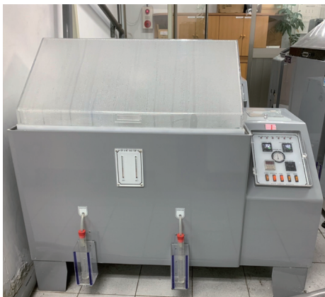
CASS 試驗機 Copper Accelerated Acetic Acid Salt Spray Tester
