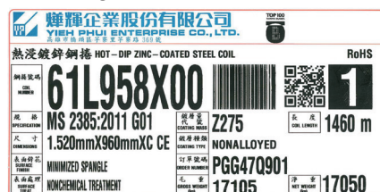
燁輝鍍鋅產品之標籤示範 Yieh Phui sample of product ID label for metallic coated steel coil
