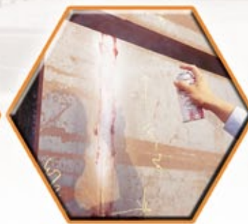
滲透探傷檢驗 Penetration Inspection
