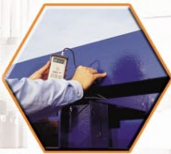
油漆膜厚檢驗 Paint Film Thickness Inspection
