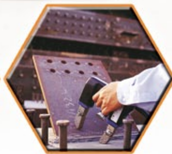
磁粉探傷檢驗 Magnetic Inspection
